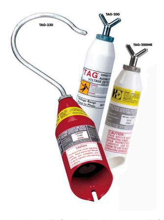
HDE's single range TAG-200, multi-range TAG-200MR and single range TAG-330 are voltage detectors designed for detecting distribution and transmission voltages. These direct contact type detectors emit both audible and visual indications when placed in contact with an energized conductor. TAG Voltage Detectors are designed for overhead and underground applications with optional underground bushing probes.
