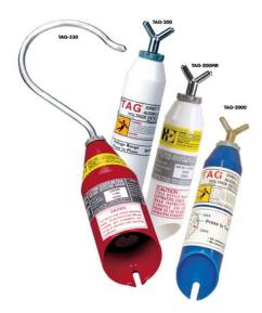
HD Electric Company's TAG Voltage Detectors are designed to detect voltage on distribution and transmission systems. When in direct contact with an energized conductor, the TAG emits an audible and visual alarm to clearly warn the user if the conductor is energized. Unlike proximity type detectors, TAG Voltage Detectors will not give false indications due to nearby energized conductors.
