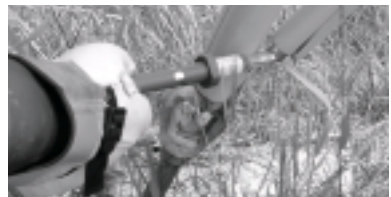
Testing anchor on a power pole.
