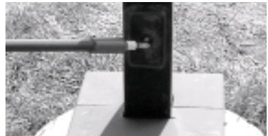
Testing street light cover with extension handle.
