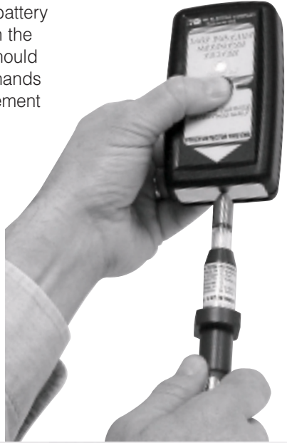
LV-S-5 Voltage Detector being used with Tester.
