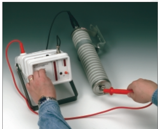
HiSat-25 testing a porcelain arrester
