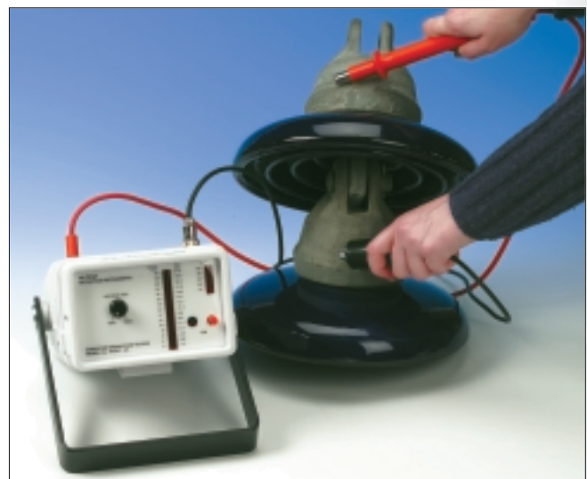
HiSat-25 testing a bell type insulator
