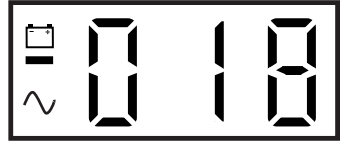
Figure 1 Low battery indicator signal shown in upper lefthand corner of display.
